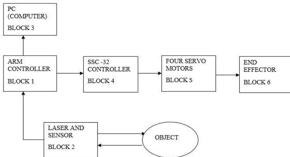
**Fig 1.1: Block diagram of the Robotic system**
