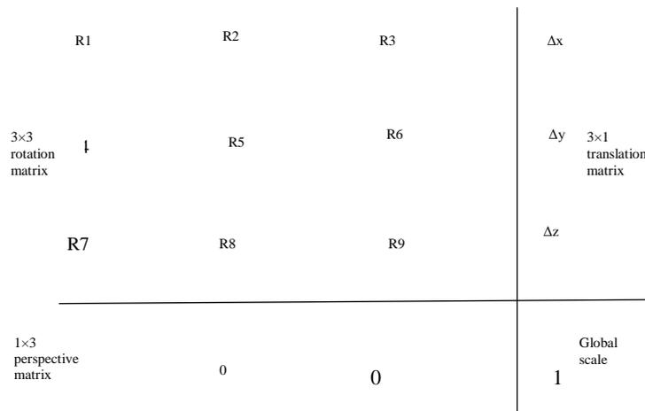
**Fig. 2.2 Homogeneous transformation matrix**
